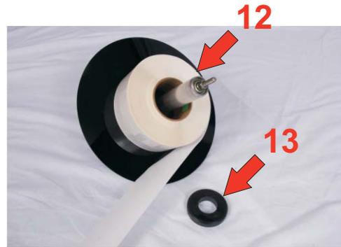
15. **Loosen** the set screws on the SIDE of the Left set collar until the washer and set collar are touching.
