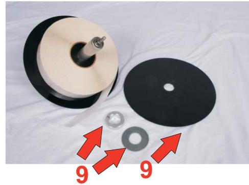
12. **Load** the desired label roll with labels coming off the roll from the bottom. The label roll should fit over the one remaining black label core adapter.
